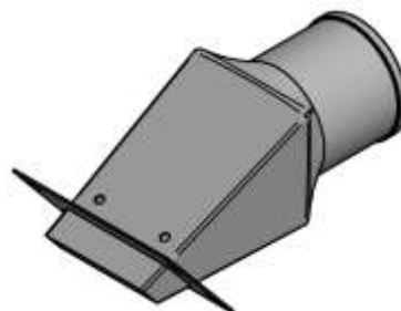
Gambar 5. Inlet Turbin Crossflow
