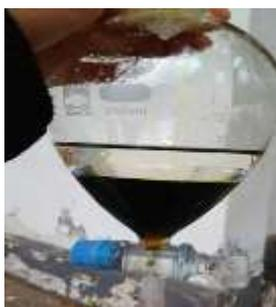
**Figure 1.** The solvent extraction solution in the glass separating funnels
