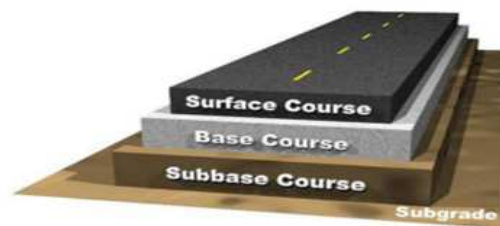
Gambar 1. Penampang Perkerasan Lentur (Widodo, 2013)
